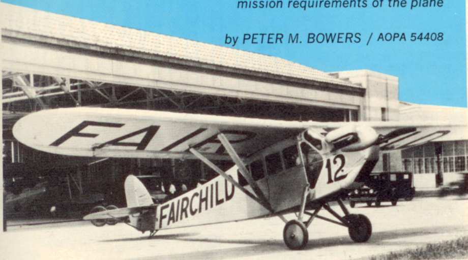
The original Fairchild FC-1, as it was flown in the Ford Air Tour of 1926. Note the neat installation of radiator under war-surplus Curtiss OX-5 engine, the full-span ailerons, and the increasing slope of the fuselage letters that indicates the triangular fuselage cross-section.
