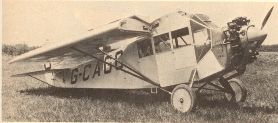
Fairchild FC-2 of 1927, with 220 h.p. Wright J-5 Whirlwind engine and folded wings. Note that the section of wing inboard of ailerons, looking like a modern flap, hinges forward over the rear spar to allow the inner portion of wing to clear the fuselage when wings are folded. Fairchild-Hiller photo
